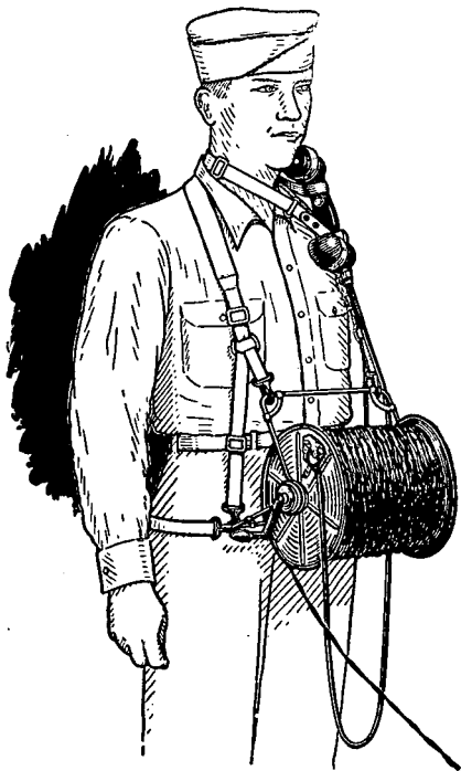
Figure 59. Reel Equipment CE-11.
